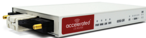
DUAL-SIM SUPPORT WITH UPGRADABLE LTE CELLULAR MODEM
