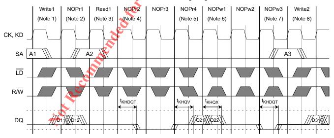
**Note**: In the diagram above, the controller is disabling its DQ ODT except from the beginning of NOPr4 to the beginning of NOPw3. And while it is disabling its DQ ODT, the controller is driving DQ Low when it isn't driving write data. Whereas, the SRAM is enabling its DQ ODT except from the beginning of NOPr2 to the beginning of NOPw3. And while it is disabling its DQ ODT, the SRAM is driving DQ Low when it isn't driving read data.
