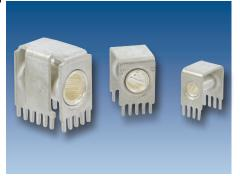
The RADSOK<sup>®</sup> PGY<sup>™</sup> provides a compact and robust right angle power to board interconnect. Designed to mate with either a 3.6mm or 5.7mm pin, The RADSOK<sup>®</sup> PGY<sup>™</sup> can bring up to 120A to the board. The radial design of the RADSOK<sup>®</sup> contact gives you more contact surface area lowering temperature rise and reducing potential heat related failures.
