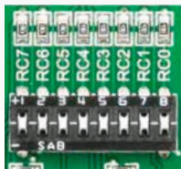
Figure 6-2: Tri-state DIP switch on PORTC
