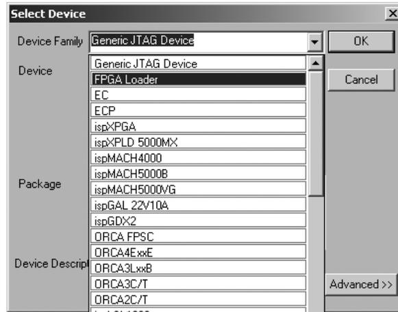
9. Use the pull-down menu to in the ‘Device Family’ field to choose the device ‘FPGA Loader’. Press OK. The resulting dialog should resemble Figure 5.
