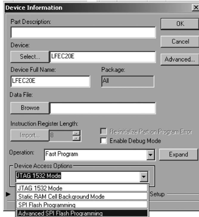
Note: Selection of the ‘Advanced SPI Flash Programming’ option allows the user to specify a data file other than the ispVM System default. This is necessary for the LatticeEC Advanced Evaluation Board.
