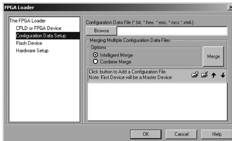
13. Click the 'Browse' button near the top of the window. Browse to the desired bitstream (.bit) file, created by the Lattice ispLEVER® design tool.
