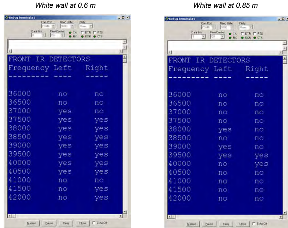
Figure 3-6 IR Receiver Frequency Response with an Object at Two Different Distances
