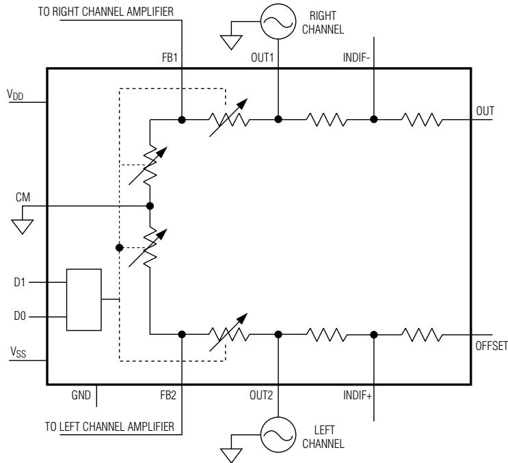
Figure 2. Stereo Audio-Taper Attenuator
