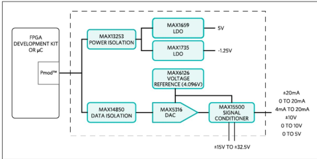
Figure 1. The Carmel subsystem design block diagram.
