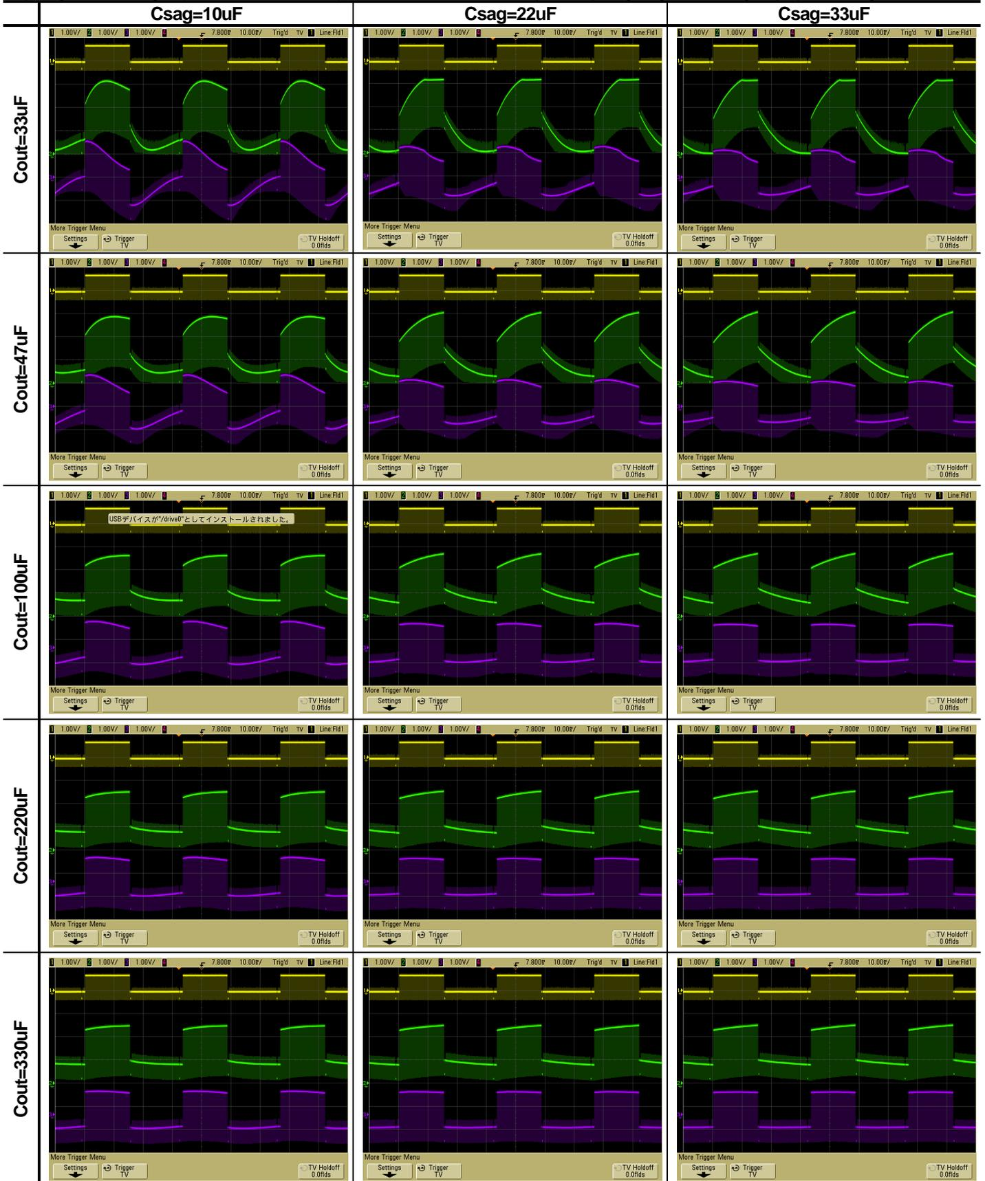
Input signal: bounce signal (IRE0%, IRE100%, 30Hz), resistance=75Ω, Waveform: yellow: input signal, green: Vout signal, purple: Vout1 signal
