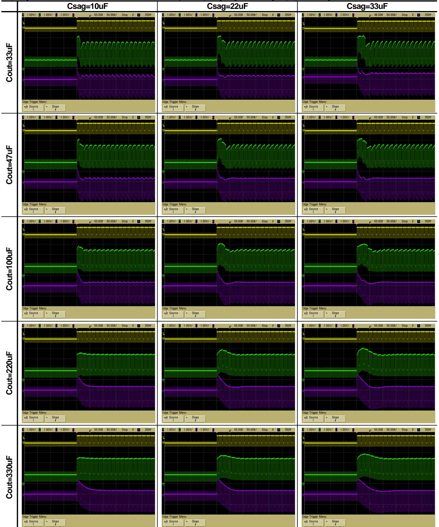
Input signal: White 100% to Black, resistance=75Ω, Waveform: yellow: input signal, green: Vout signal, purple: Vout1 signal
