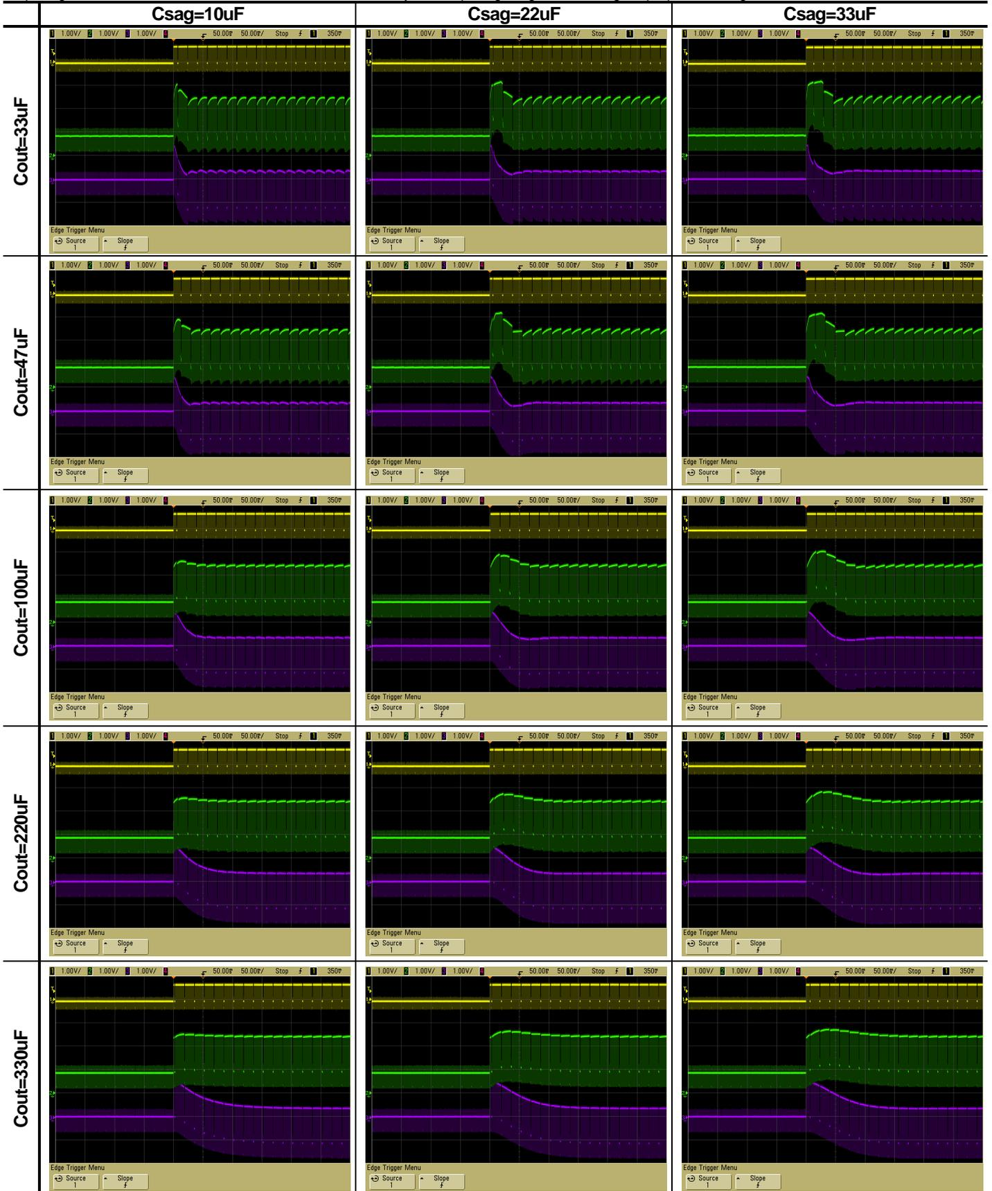
Input signal: White 100% to Black, resistance 150Ω, Waveform: yellow: input signal, green: Vout signal, purple: Vout1 signal
