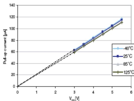
**Figure 24. Typical pull-up resistance vs  $V_{DD}$  @ 4 temperatures**
