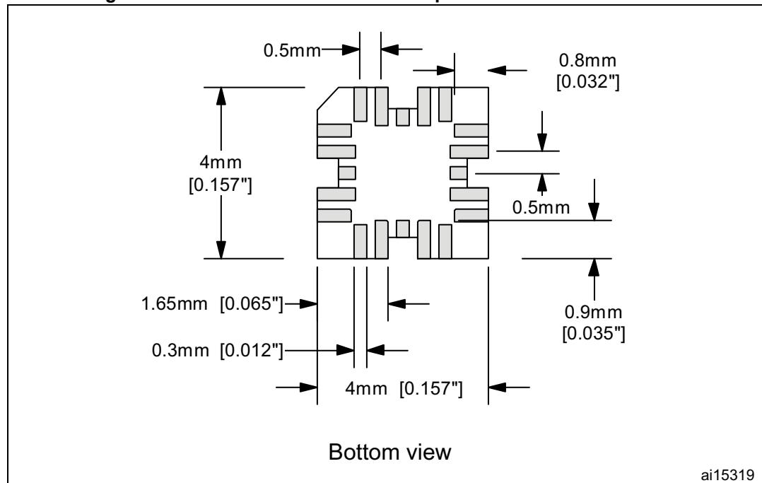
**Figure 62. UFQFPN recommended footprint without on-board emulation**
