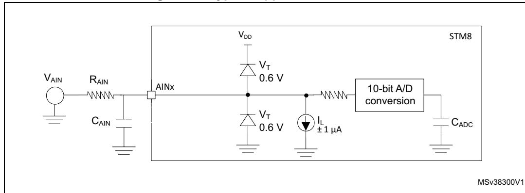
1. Legend:  $R_{AIN}$  = external resistance,  $C_{AIN}$  = capacitors,  $C_{samp}$  = internal sample and hold capacitor.
