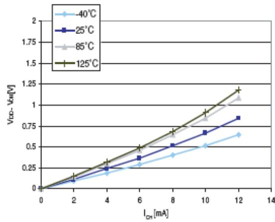
**Figure 34. Typ.  $V_{DD} - V_{OH}$  @  $V_{DD} = 5.0$  V (high sink ports)**
