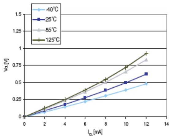
**Figure 30. Typ.  $V_{OL}$  @  $V_{DD} = 5.0$  V (high sink ports)**
