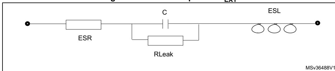
1. ESR is the equivalent series resistance and ESL is the equivalent inductance.
