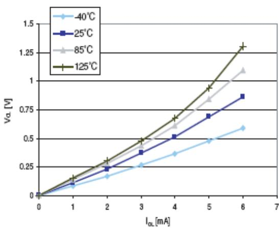
**Figure 26. Typ.  $V_{OL}$  @  $V_{DD} = 5.0 \text{ V}$  (standard ports)**
