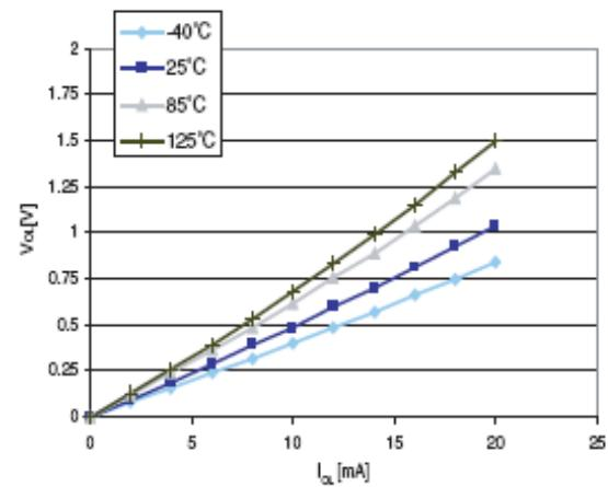
**Figure 29. Typ.  $V_{OL}$  @  $V_{DD} = 3.3$  V (high sink ports)**
