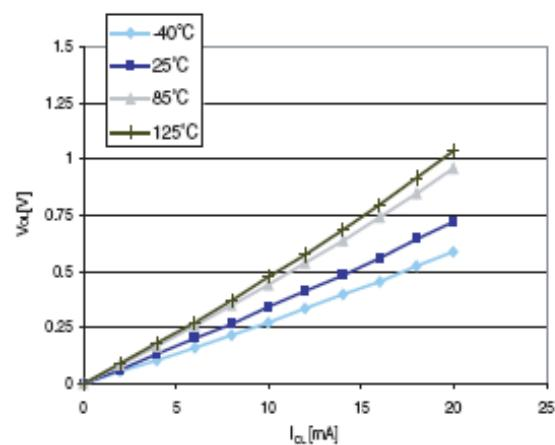
**Figure 31. Typ.  $V_{DD} - V_{OH}$  @  $V_{DD} = 3.3$  V
