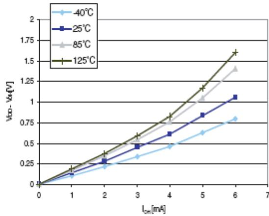
**Figure 32. Typ.  $V_{DD} - V_{OH}$  @  $V_{DD} = 5.0$  V
