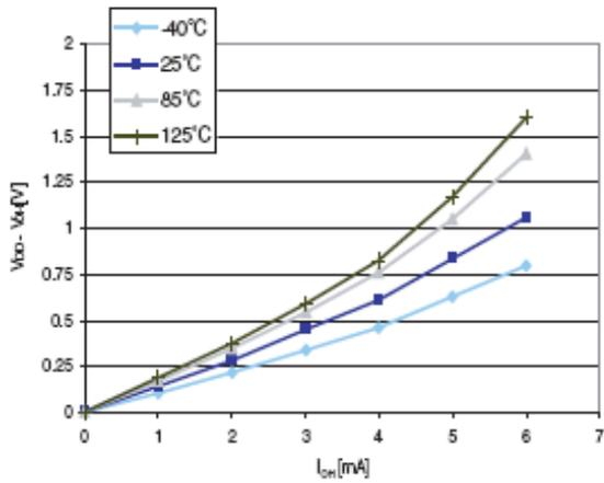
Figure 32. Typ.  $V_{DD} - V_{OH}$  @  $V_{DD} = 5.0\text{ V}$  (standard ports)
