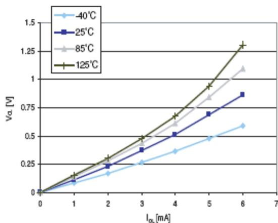
**Figure 26. Typ. V<sub>OL</sub> @ V<sub>DD</sub> = 5.0 V (standard ports)**
