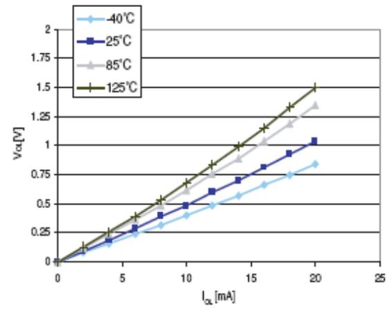
Figure 29. Typ.  $V_{OL}$  @  $V_{DD} = 3.3$  V (high sink ports)
