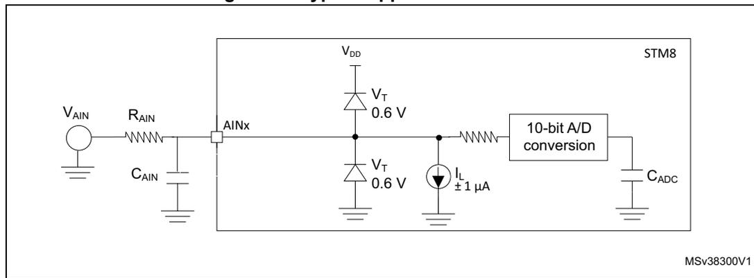
1. Legend:  $R_{AIN}$  = external resistance,  $C_{AIN}$  = capacitors,  $C_{s\text{amp}}$  = internal sample and hold capacitor.
