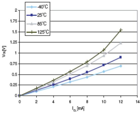
Figure 28. Typ.  $V_{OL}$  @  $V_{DD} = 5.0$  V (true open drain ports)
