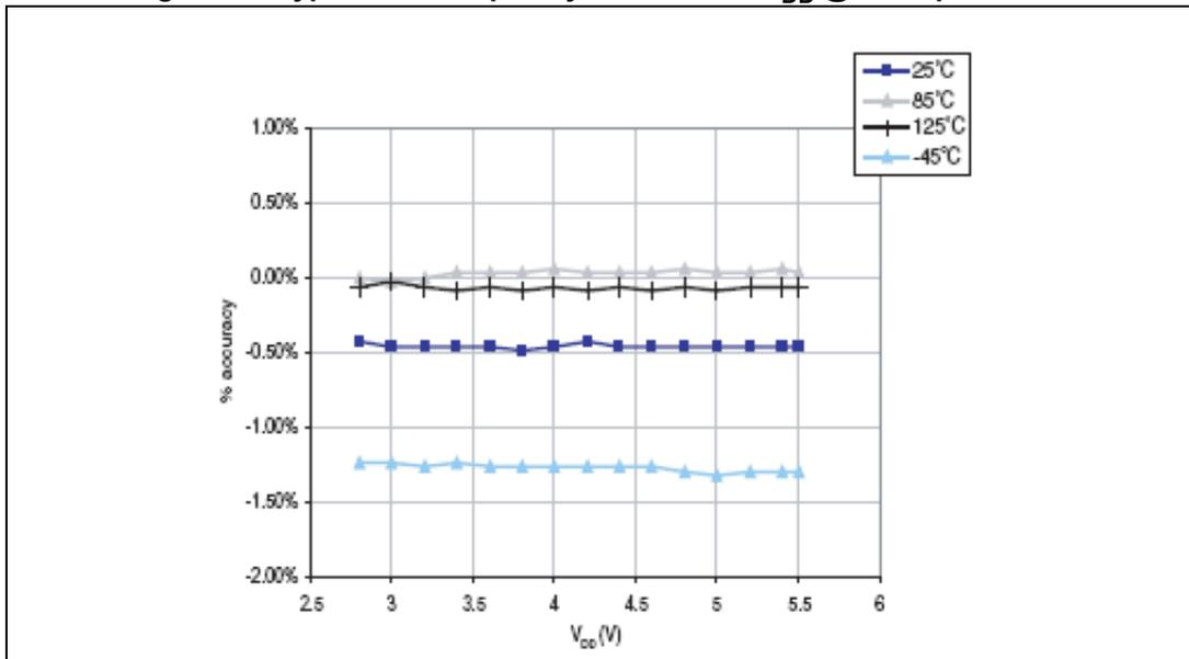
**Low speed internal RC oscillator (LSI)**
