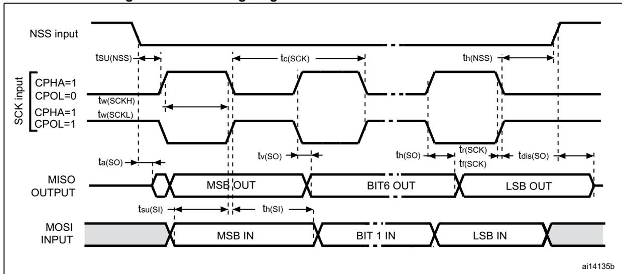
1. Measurement points are at CMOS levels: 0.3  $V_{DD}$  and 0.7  $V_{DD}$ .
