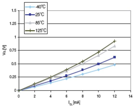
Figure 30. Typ.  $V_{OL}$  @  $V_{DD} = 5.0$  V (high sink ports)
