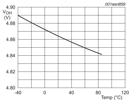
**Fig 10. HIGH-level output voltage versus temperature**
