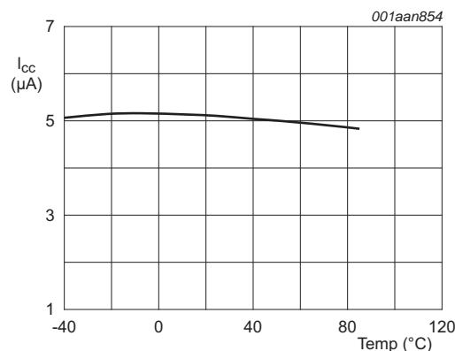
**Fig 5. Supply current versus temperature**
