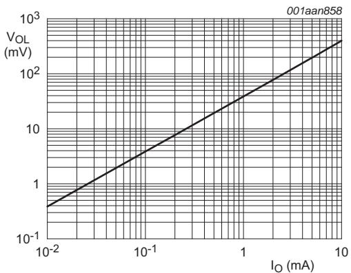
**Fig 9. LOW-level output voltage versus output current**
