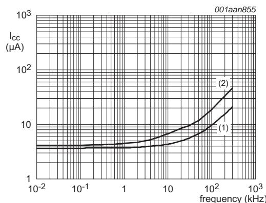
**Fig 6. Supply current versus output transition frequency**
