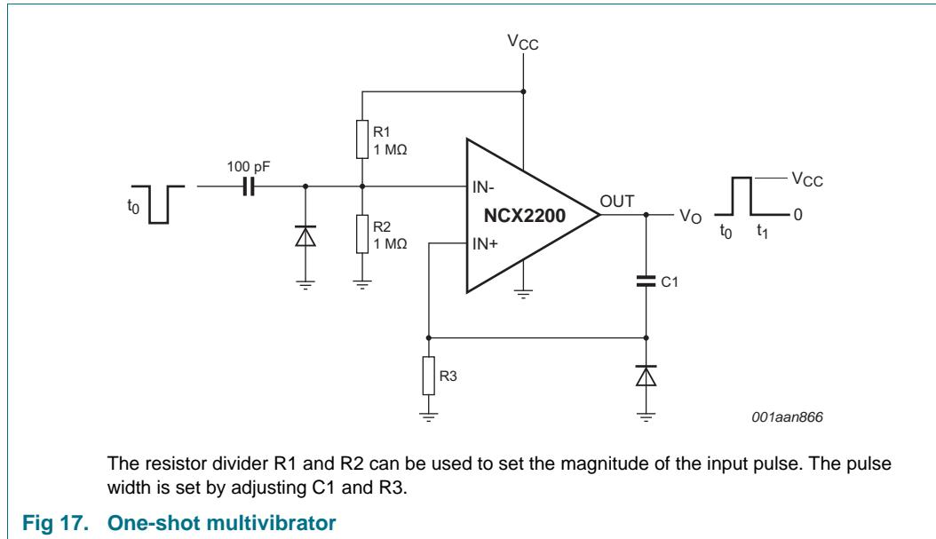
The resistor divider  $R_1$  and  $R_2$  can be used to set the magnitude of the input pulse. The pulse width is set by adjusting  $C_1$  and  $R_3$ .
