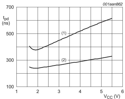
$T_{amb} = 25 \text{ °C}$ ; input overdrive = 100 mV.
