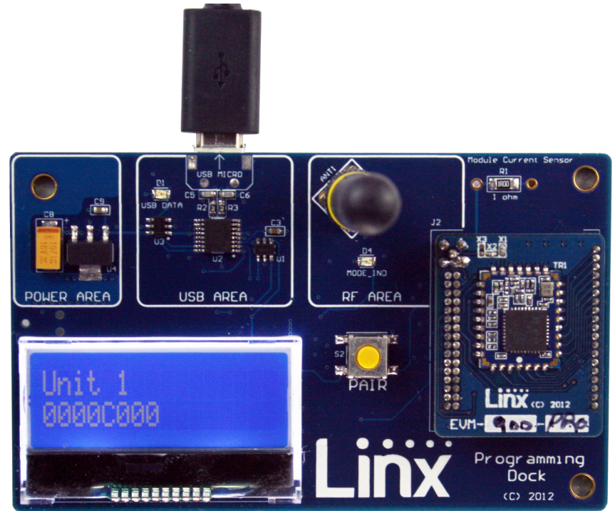
Figure 13: The Master Development System Programming Dock with Name and Address Displayed
