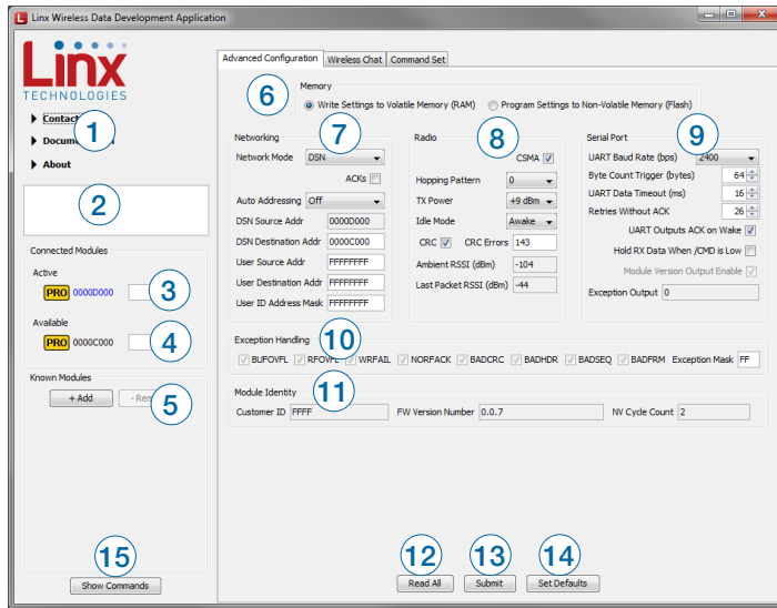
Figure 10: The Master Development System Software Advanced Configuration Tab
