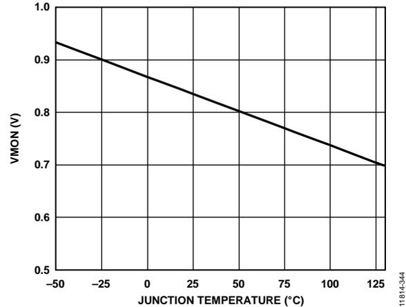
Figure 9. V<sub>MON</sub> Output Voltage vs. Junction Temperature  $V_{MON} (V) = -0.0013 \times TEMP(C) + 0.8675$
