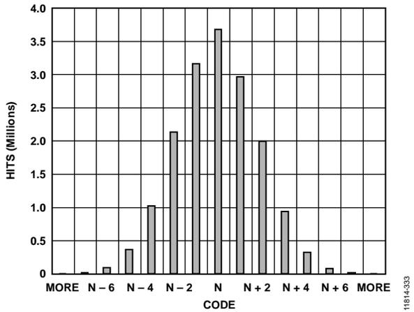
Figure 38. Input Referred Noise Histogram with 2.5 GSPS
