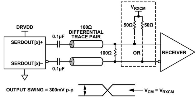
Figure 89. AC-Coupled Digital Output Termination Example
