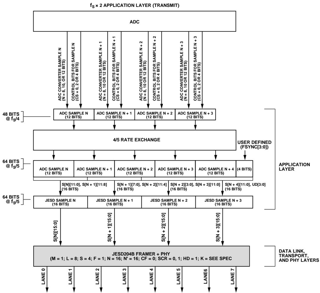
Figure 104.  $f_s \times 2$  Mode Application Layer (Transmit)
