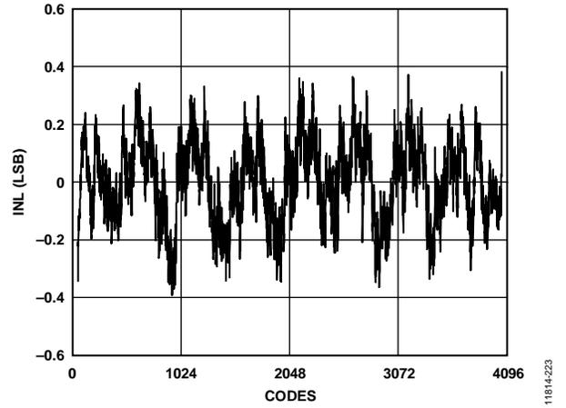
Figure 24. Integral Nonlinearity (INL),  $\pm 0.4$  LSB at 2.0 GSPS
