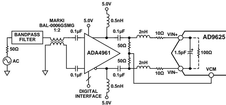
Figure 80. Configuration for Driving the AD9625 with ADA4961
