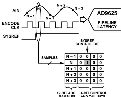
Figure 95. A SYSREF± Control Bit Can Be Used to Mark the Same Analog Sample that is Coincident with a Sampled SYSREF± Edge by CLK±
