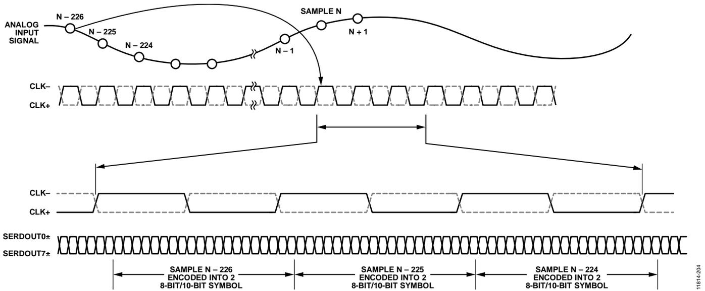
Figure 4. Data Output Timing for Eight Lane Mode
