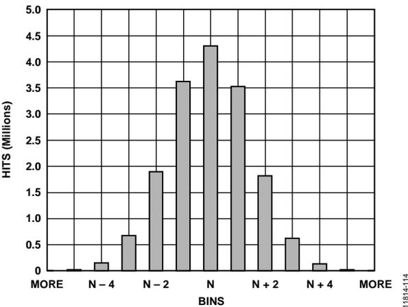
Figure 18. Input Referred Noise Histogram with 2.0 GSps
