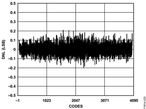
Figure 23. Differential Nonlinearity (DNL),  $\pm 0.2$  LSB at 2.0 GSPS
