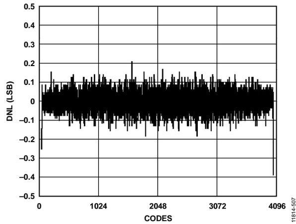
Figure 59. Differential Nonlinearity (DNL) at 2.6 GSPS
