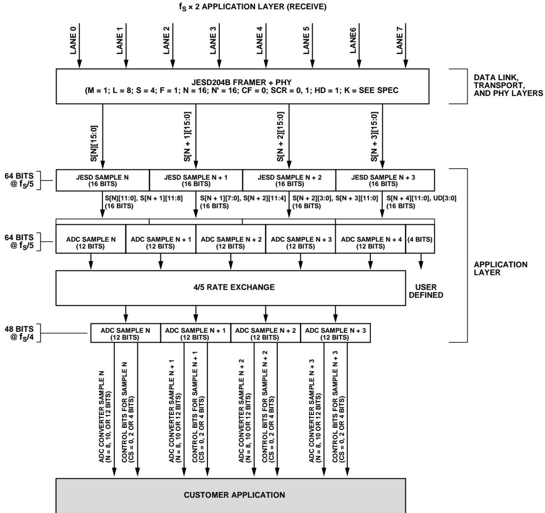
Figure 105.  $f_s \times 2$  Application Layer (Receive)
