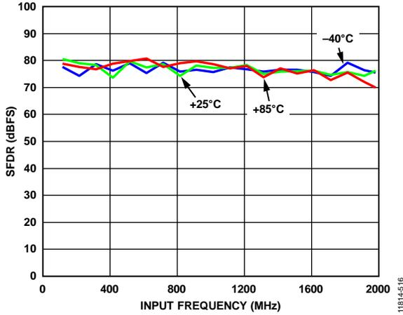
Figure 51. SFDR vs. Temperature at 2.6 GSPS
