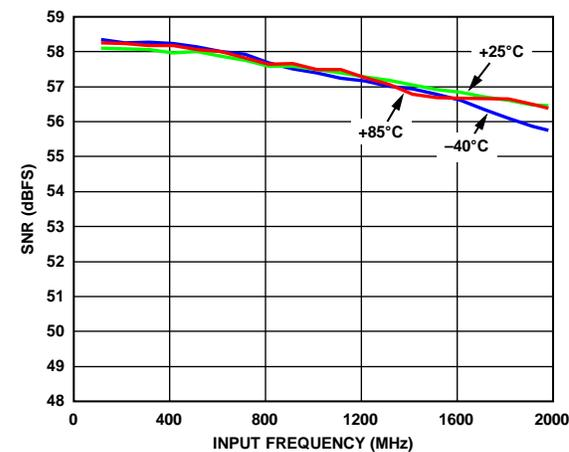
Figure 50. SNR vs. Temperature at 2.6 GSPS
