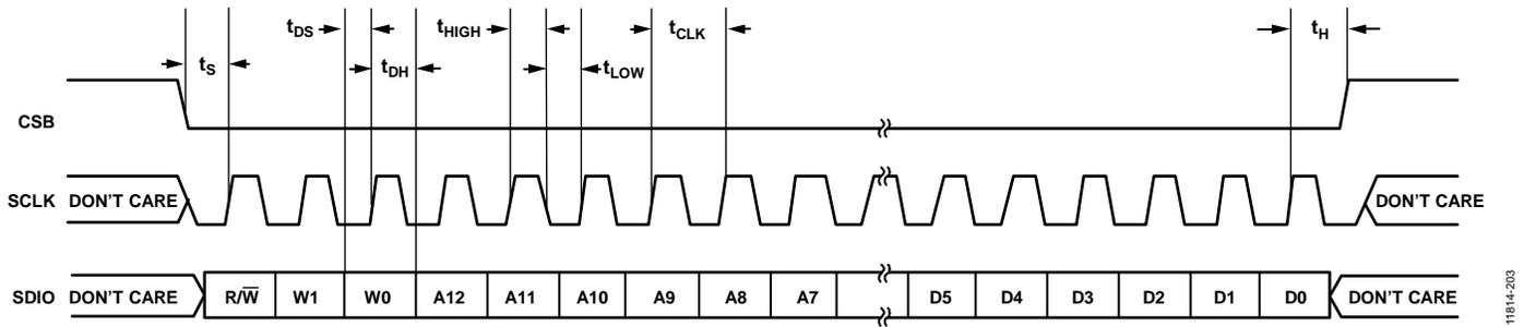
Figure 3. Serial Port Interface Timing Diagram (MSB First)
