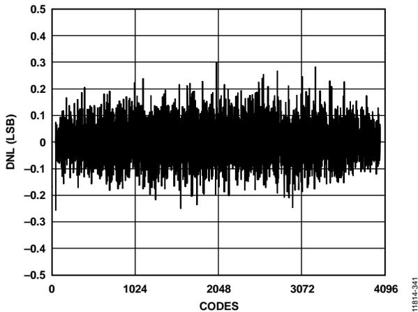
Figure 39. Differential Nonlinearity (DNL),  $\pm 0.3$  LSB at 2.5 GSPS
