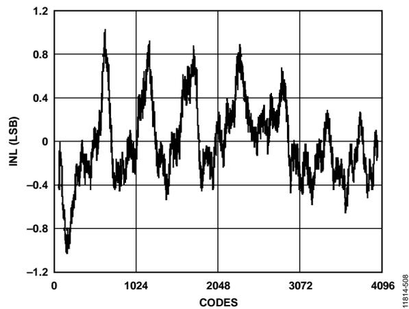
Figure 60. Integral Nonlinearity (INL) at 2.6 GSPS
