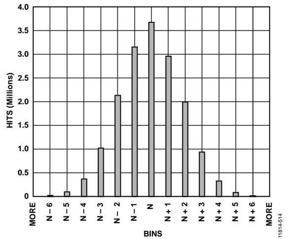
Figure 55. Input Referred Noise Histogram with 2.6 GSPS
