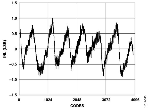
Figure 44. Integral Nonlinearity (INL),  $\pm 1.0$  LSB at 2.5 GSPS
