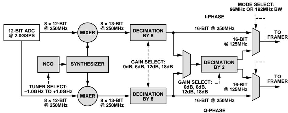
Figure 82. Digital Downconverter Block Diagram Operating at 2.0 GSPS
