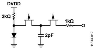
Figure 63. Equivalent VMON Temperature Sensor Circuit (DVDD)
