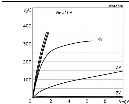
**Figure 5. Transfer characteristics**
