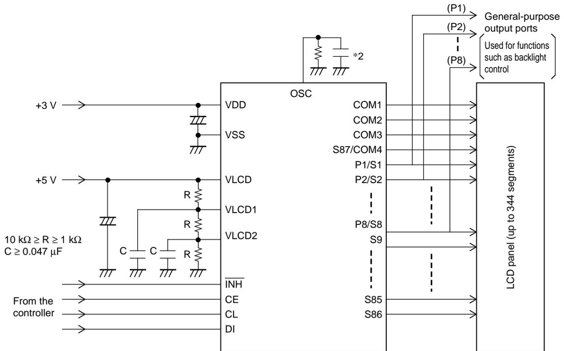
Note: \*2 When a capacitor except the recommended external capacitance ( $C_{osc} = 1000 \text{ pF}$ ) is connected the OSC pin, we recommend that applications connect the OSC pin with a capacitor in the range 220 to 2200 pF.
