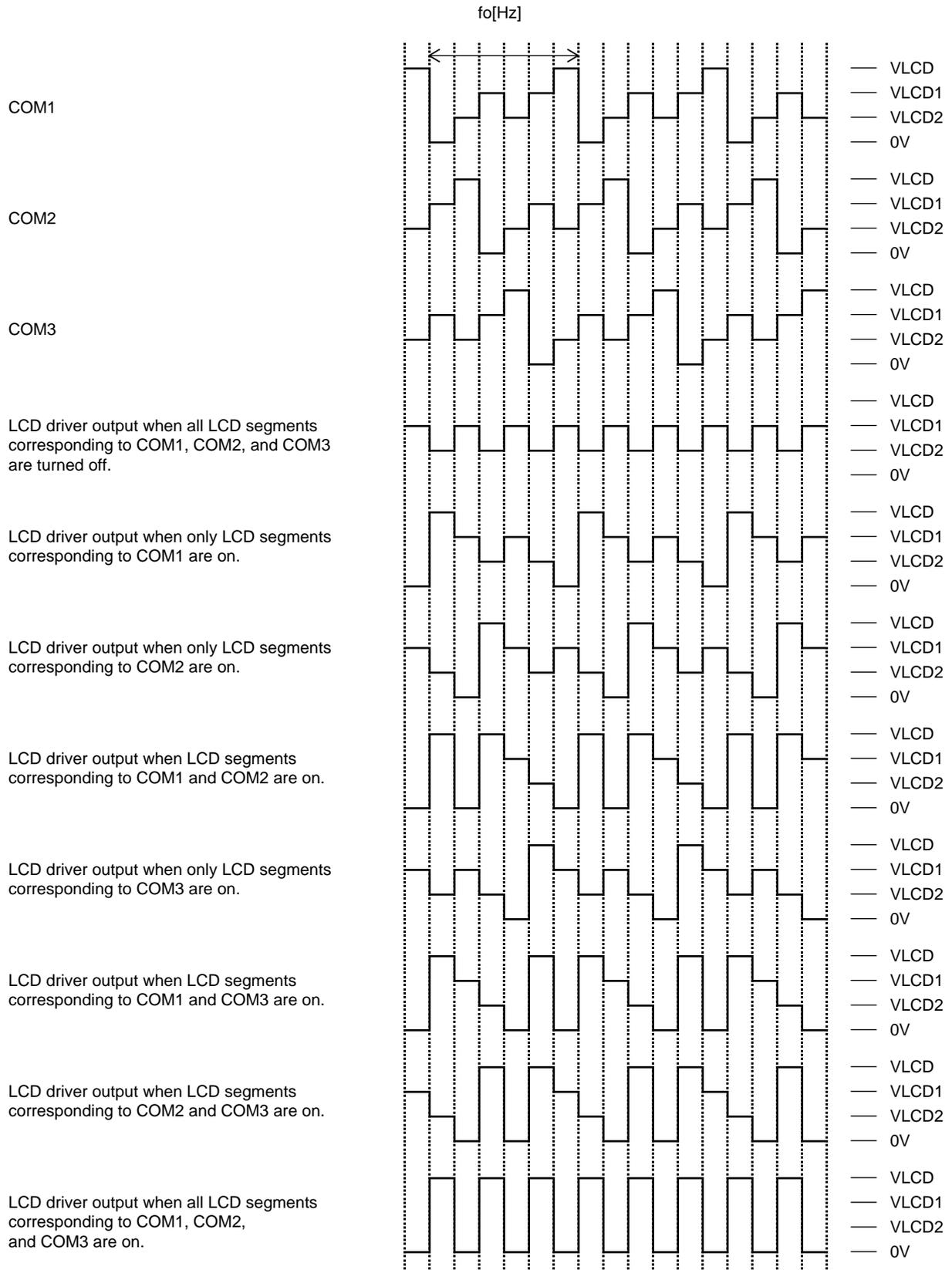
$$\left( \begin{array}{l} \text{When the control data FC} = 0 : f_o = \frac{f_{osc}}{384} \\ \text{When the control data FC} = 1 : f_o = \frac{f_{osc}}{192} \end{array} \right)$$
