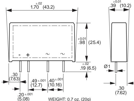
*Figure 1 – BS relays; dimensions in inches (mm)*
