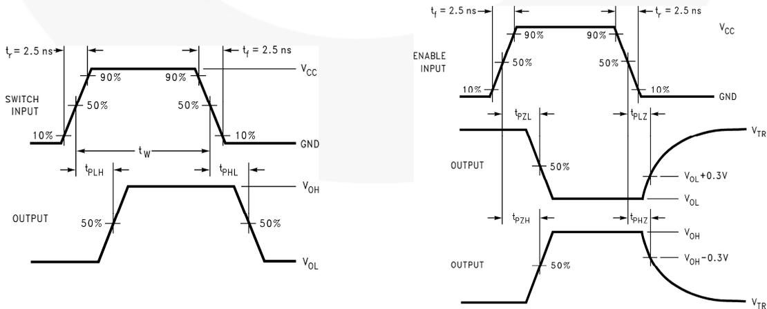
Figure 5. AC Waveforms
