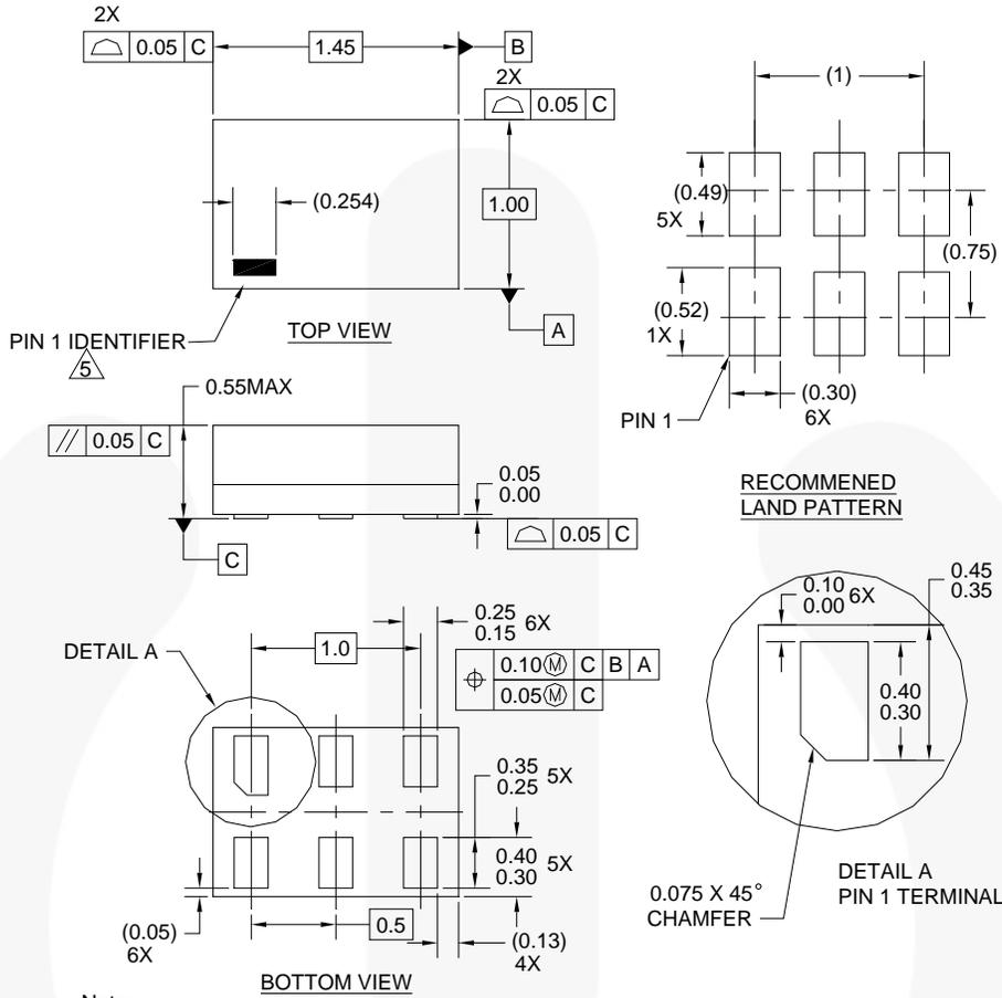
**Figure 8. 6-Lead, MicroPak™, 1.0 mm Wide**
