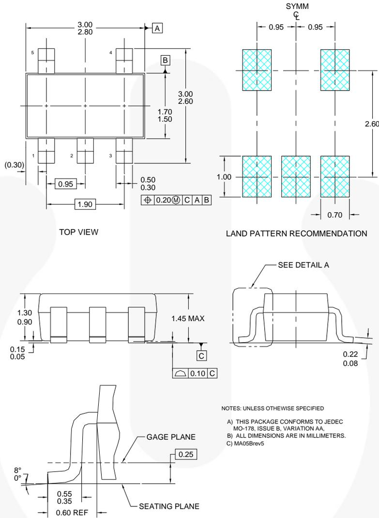
**Figure 6. 5-Lead SOT23, JEDEC MO-178 1.6 mm**
