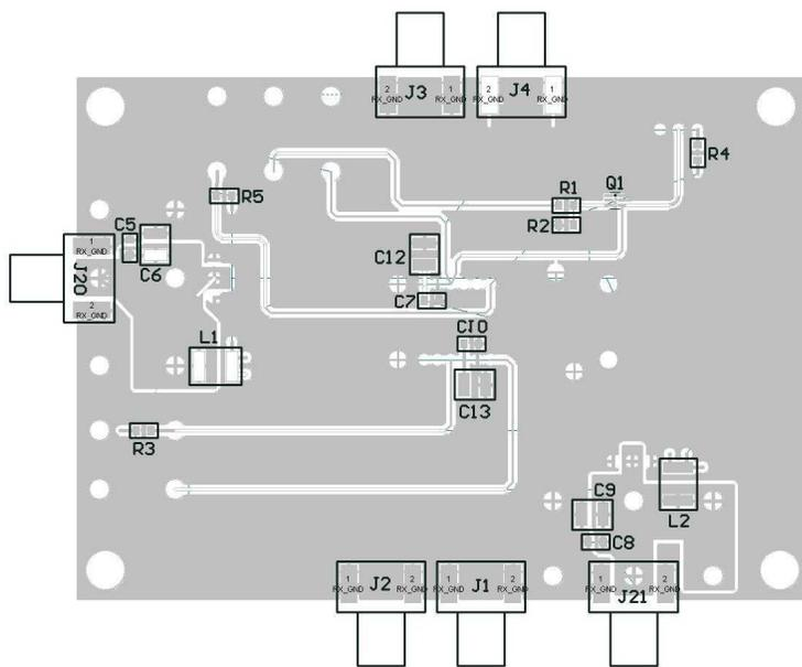
Figure 1. SFF Evaluation Board Top and Bottom View
