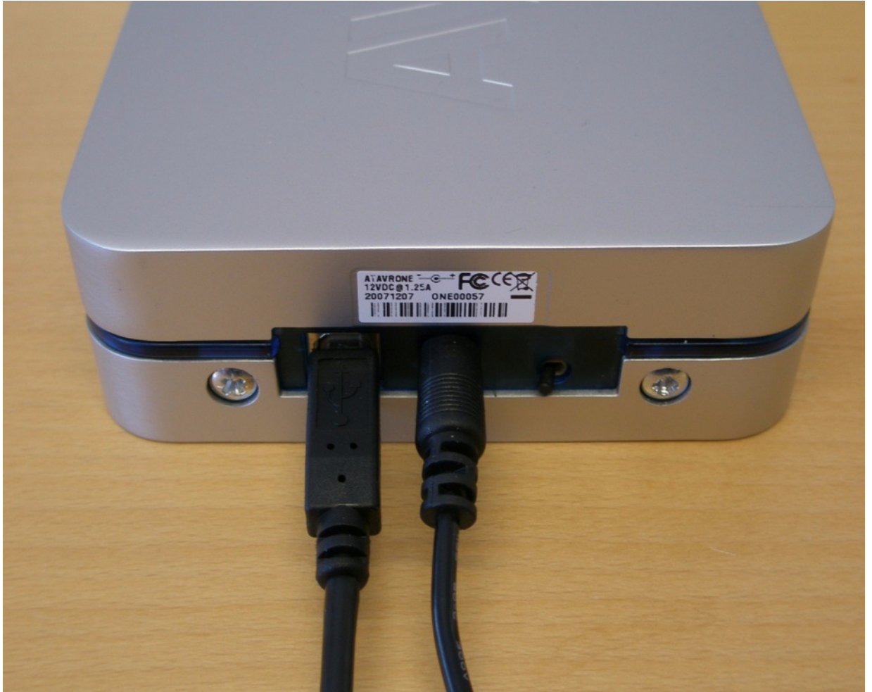
Figure 4-19. AVR ONE! connected to power and USB
