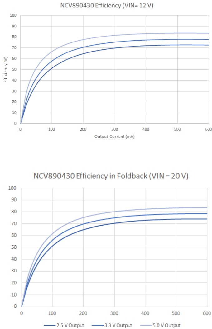
Figure 6. NCV890430 Efficiency Curves
