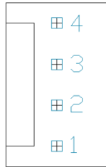
Figure 12: I 2 C Communication/Power Header
