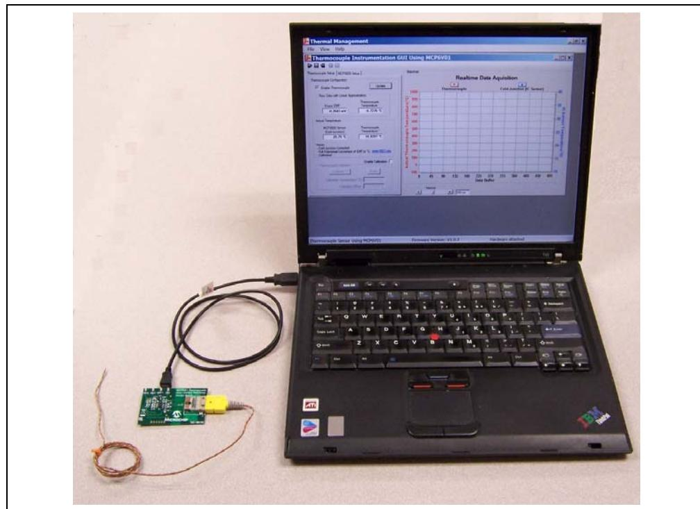
**FIGURE 2-1:** MCP6V01 Thermocouple Auto-Zeroed Reference Design Setup.
