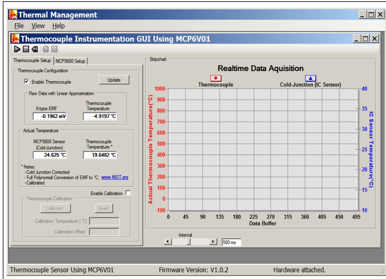
**FIGURE 2-5:** Thermocouple setup.
