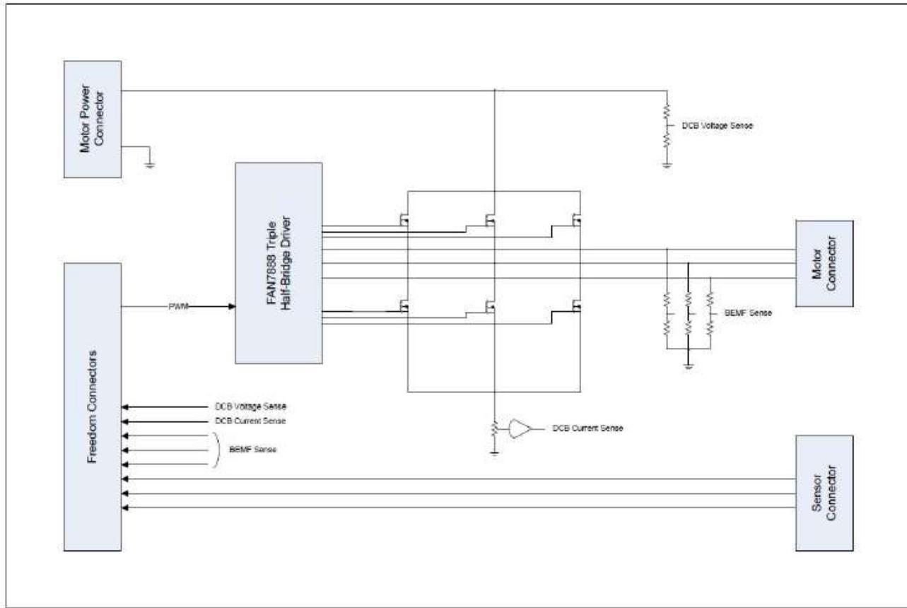
**Figure 1. FRDM-MC-LVPMSM platform block diagram**
