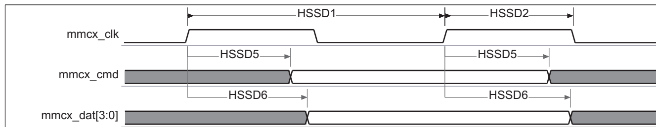
Figure 6-65. MMC/SD/SDIO – High-Speed SD Mode – Data/Command Receive
