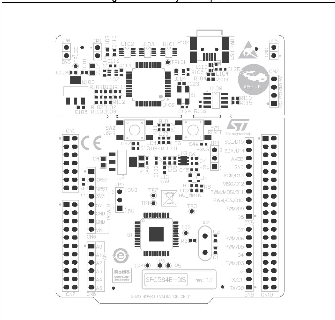
**Figure 15. PCB Layout - Bottom Side**
