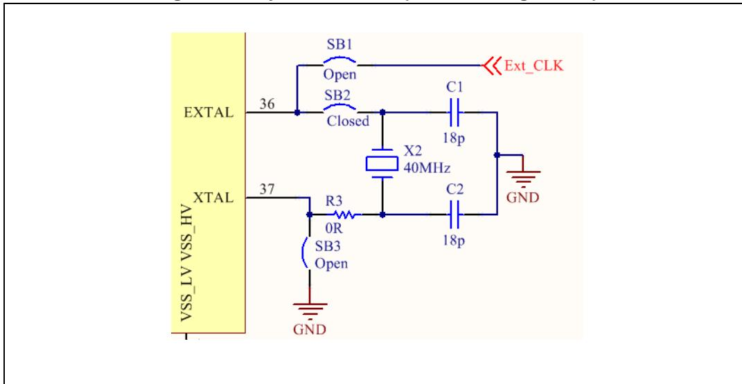
The jumpers SB1, SB2 and SB3 allow enabling further input clock as described in [Table 3](#).
