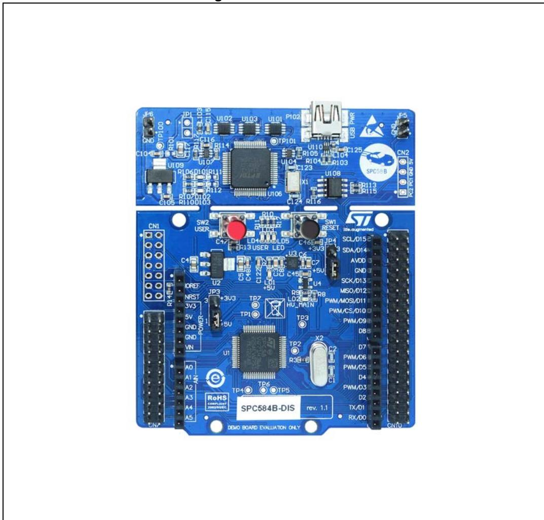
The board integrates a PLS programmer/debugger that allows debugging and programming the microcontroller via USB cable. In addition, it allows enabling a USART communication channel (USB Virtual COM port).
