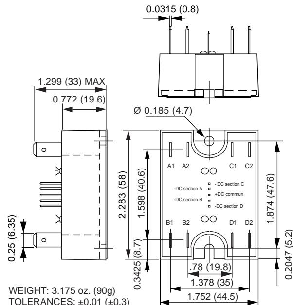
Figure 1 — SQ relay; dimensions in inches (mm)
