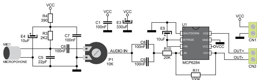
Figure 2: MICROPHONE AMP additional board connection schematic
