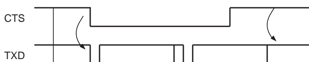
Figure 44-28. Transmitter Behavior when Operating with Hardware Handshaking
