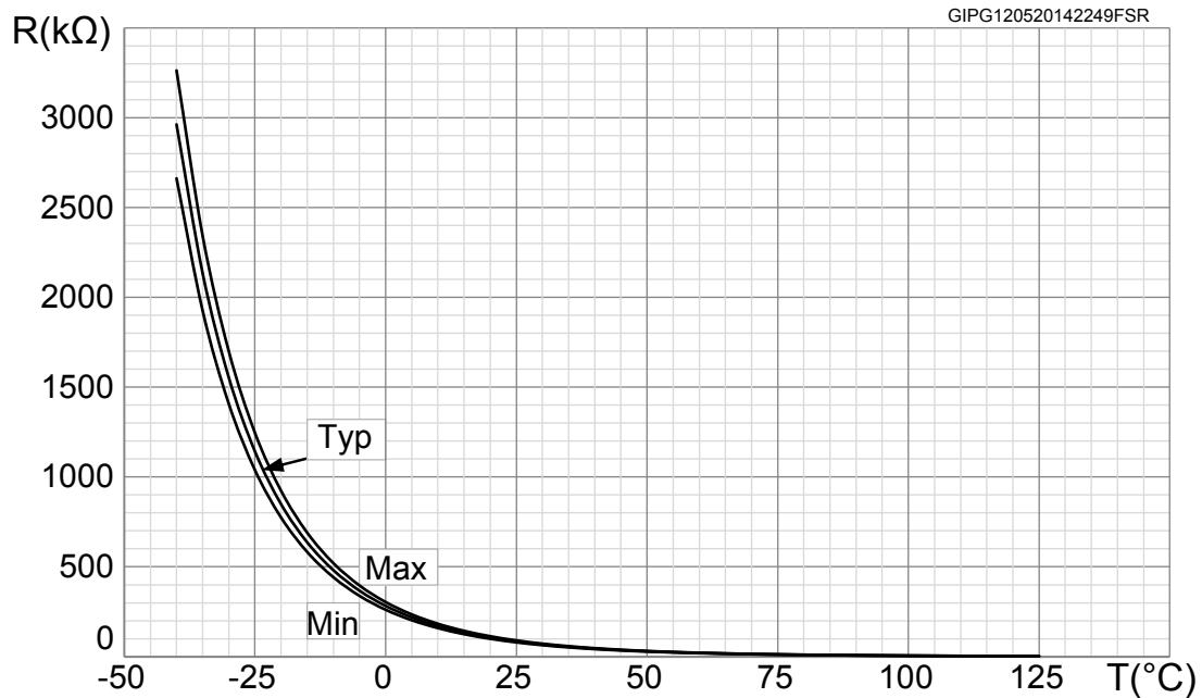
**Figure 9.** NTC resistance vs temperature - zoom
