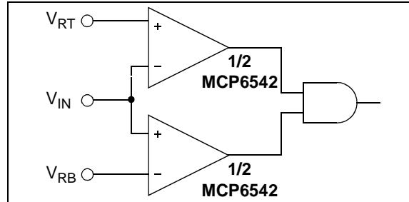
**FIGURE 4-12:** Windowed Comparator.
