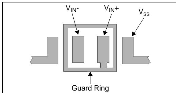
**FIGURE 4-9:** Example Guard Ring Layout for Inverting Circuit.
