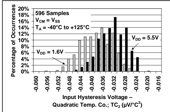
**FIGURE 2-6:** Input Hysteresis Voltage – Quadratic Temp. Co. (TC<sub>2</sub>) at  $V_{CM} = V_{SS}$ .
