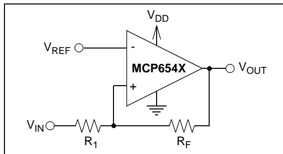
**FIGURE 4-4:** Non-inverting Circuit with Hysteresis for Single-supply.
