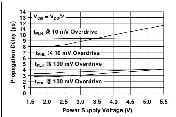
**FIGURE 2-26:** Propagation Delay vs. Power Supply Voltage.
