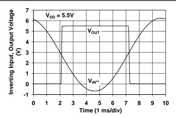
**FIGURE 2-3:** The MCP6541/1R/1U/2/3/4 Comparators Show No Phase Reversal.
