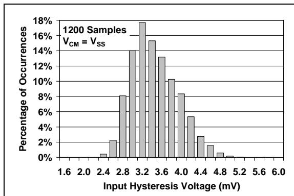
**FIGURE 2-4:** Input Hysteresis Voltage at  $V_{CM} = V_{SS}$ .
