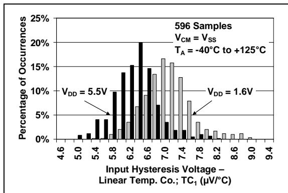
**FIGURE 2-5:** Input Hysteresis Voltage – Linear Temp. Co. (TC<sub>1</sub>) at  $V_{CM} = V_{SS}$ .
