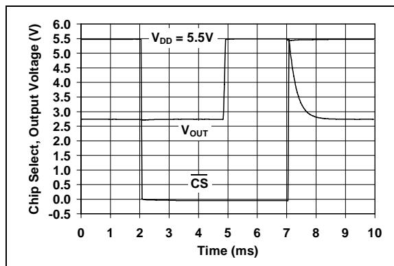
FIGURE 2-34: Chip Select (CS) Step Response (MCP6543 only).
