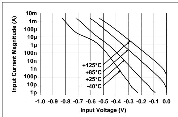
**FIGURE 2-37:** Input Bias Current vs. Input Voltage.
