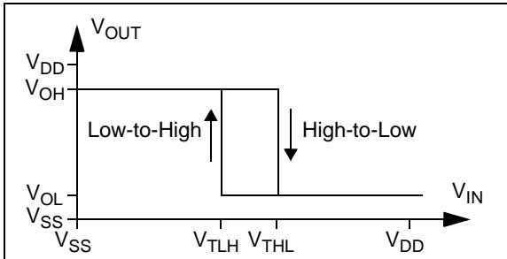
**FIGURE 4-7:** Hysteresis Diagram for the Inverting Circuit.
