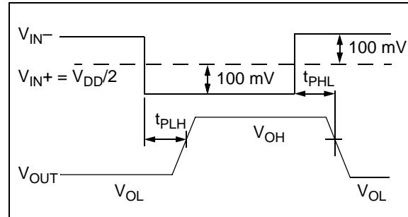
**FIGURE 1-2:** Propagation Delay Timing Diagram.
