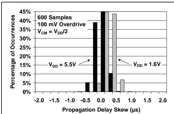
**FIGURE 2-25:** Propagation Delay Skew.
