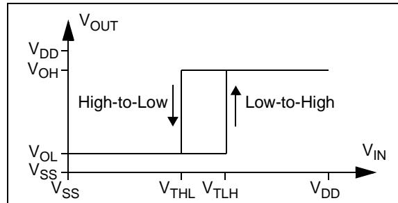
**FIGURE 4-5:** Hysteresis Diagram for the Non-Inverting Circuit.
