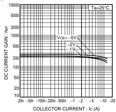
Fig.2 DC current gain vs. collector current ( I )
