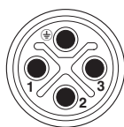
M12 plug pin assignment, 4-pos., S-coded, plug side view
