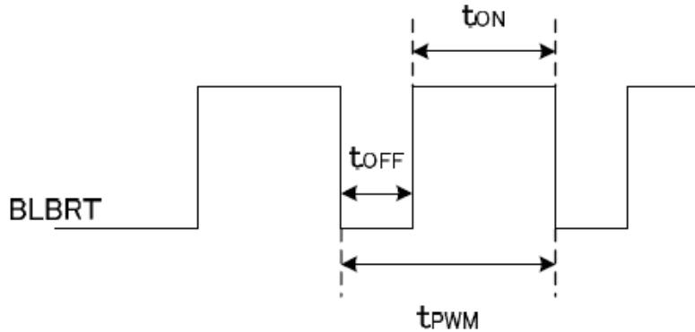
$t_{ON}, t_{OFF} \geq 50 \mu s$ .
