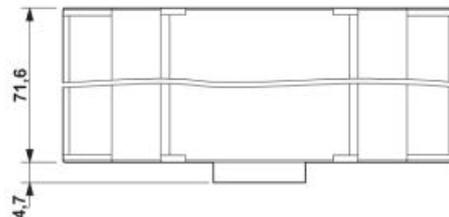
The dimensional drawing shows the item along with the lower part of the housing (terminal installation depth 11.1 mm) and the housing cover
