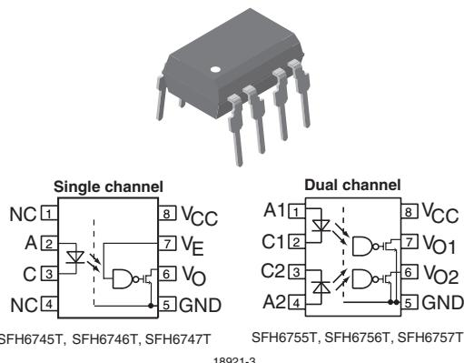
For the single channel type, an enable function on pin 7 allows the detector to be strobed. The internal shield provides a guaranteed common mode transient immunity of 5 kV/μs for the SFH6741 and SFH6751 and 10 kV/μs for the SFH6742 and SFH6752. The use of a 0.1 μF bypass capacitor connected between pin 5 and 8 is recommended.
