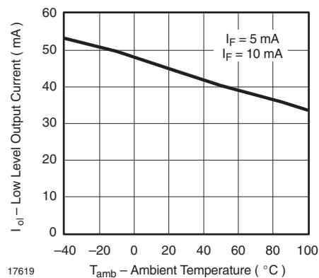
Figure 14. Low Level Output Current vs. Ambient Temperature
