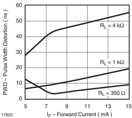
Figure 20. Pulse Width Distortion vs. Forward Current
