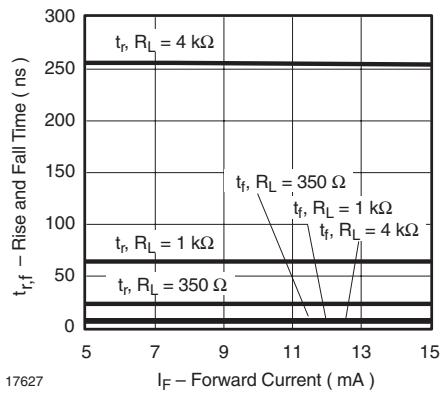
Figure 22. Rise and Fall Time vs. Forward Current
