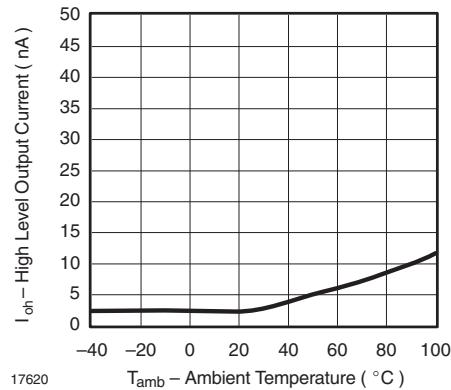
Figure 15. High Level Output Current vs. Ambient Temperature
