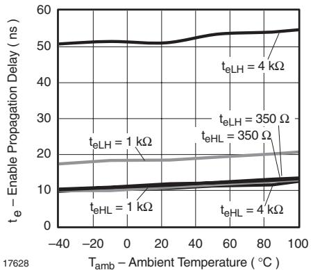
Figure 23. Enable Propagation Delay vs. Ambient Temperature
