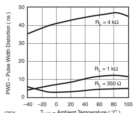
Figure 19. Pulse Width Distortion vs. Ambient Temperature
