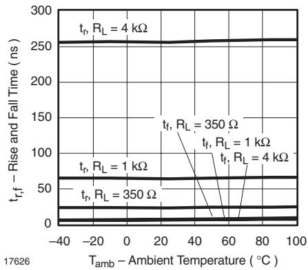
Figure 21. Rise and Fall Time vs. Ambient Temperature
