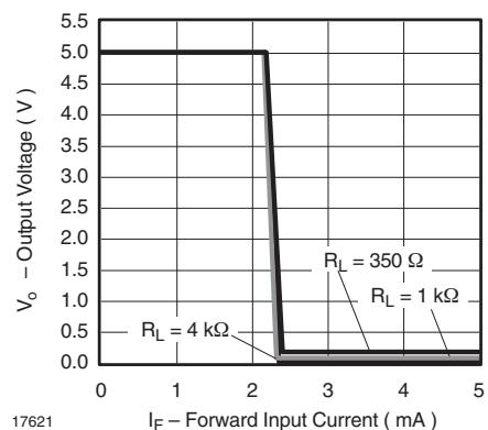
Figure 16. Output Voltage vs. Forward Input Current
