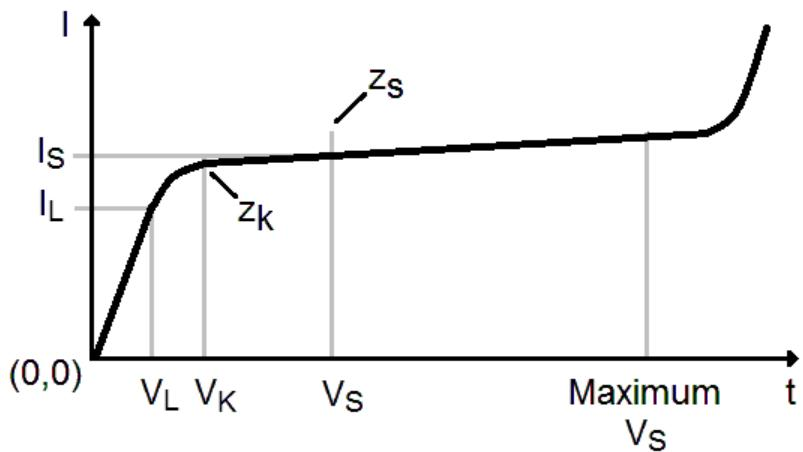
**FIGURE 1 – CURRENT-REGULATOR CHARACTERISTICS**
