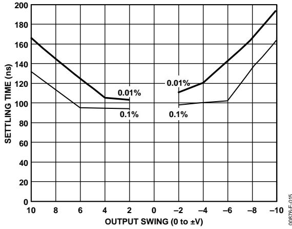
Figure 17. Output Swing and Error vs. Settling Time
