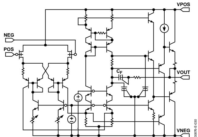
Figure 32. Simplified Schematic
