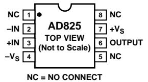
Figure 1. 8-Lead Plastic SOIC (R-8) Package
