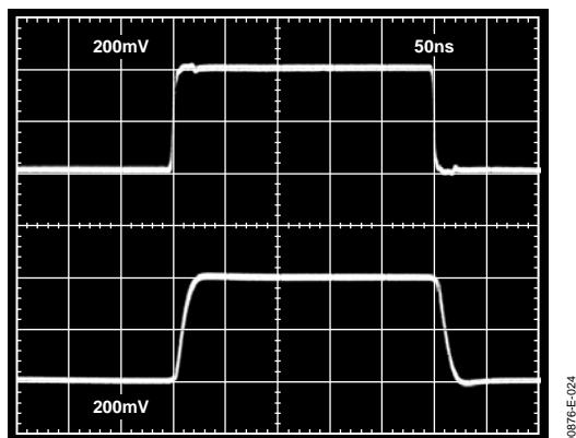
Figure 26. Noninverting Small Signal Pulse Response,  $R_L = 150 \Omega$
