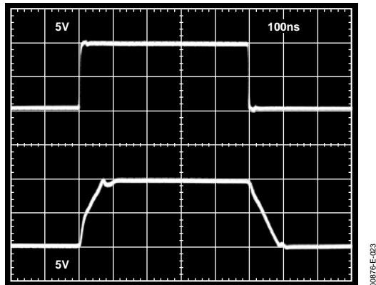
Figure 25. Noninverting Large Signal Pulse Response,  $R_L = 150 \Omega$
