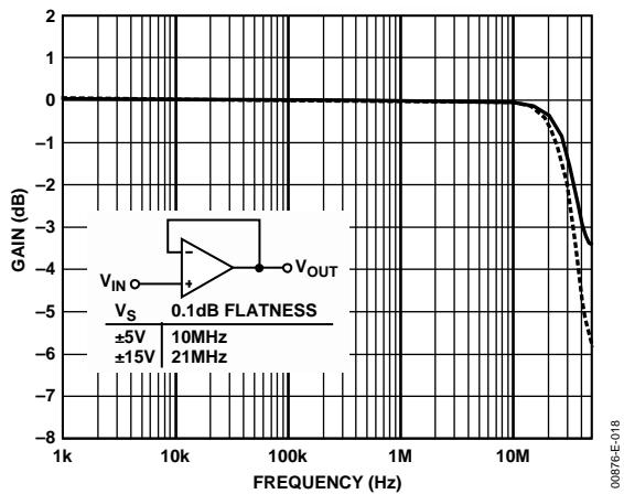
Figure 20. Closed-Loop Gain vs. Frequency, Gain = +1
