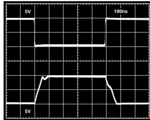
Figure 28. Inverting Large Signal Pulse Response,  $R_L = 1 k\Omega$
