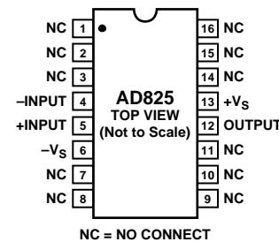
Figure 2. 16-Lead Plastic SOIC (RW-16) Package
