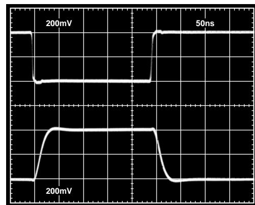
Figure 29. Inverting Small Signal Pulse Response,  $R_L = 1 k\Omega$
