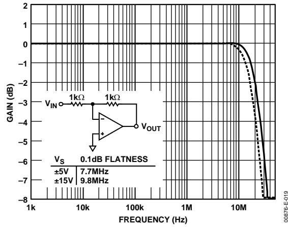
Figure 21. Closed-Loop Gain vs. Frequency, Gain = -1
