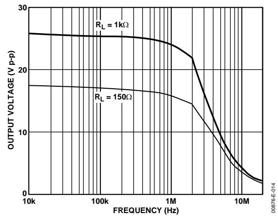
Figure 16. Large Signal Frequency Response;  $G = +2$
