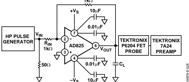
Figure 30. Inverting Amplifier Driving a Capacitive Load
