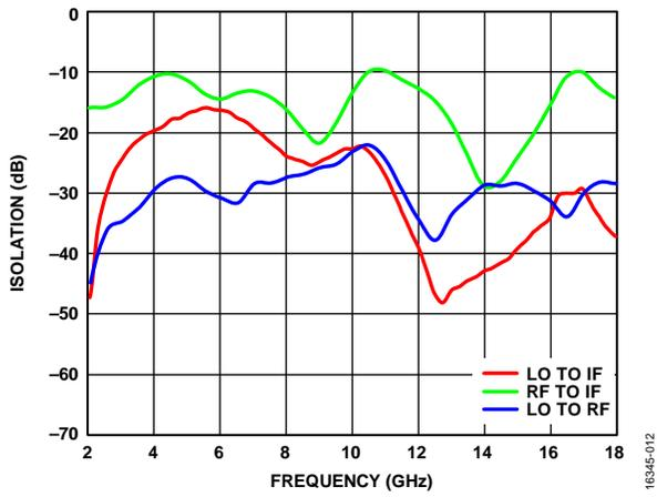
Figure 26. Isolation vs. Frequency,  $T_A = 25^\circ\text{C}$
