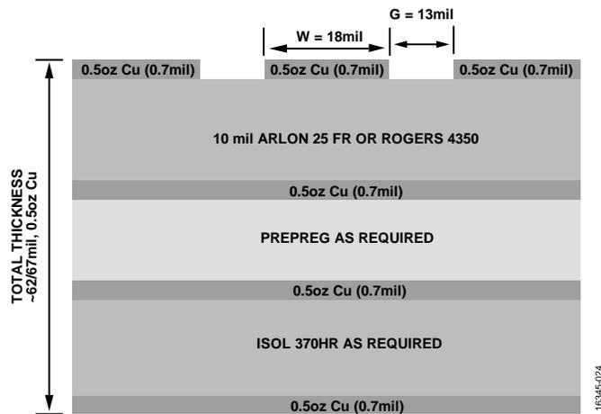
Figure 31. EV1HMC1048ALC3B Evaluation Board Cross Sectional View
