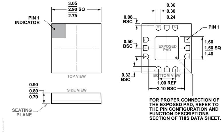
Figure 34. 12-Terminal Ceramic Leadless Chip Carrier [LCC] (E-12-4)
