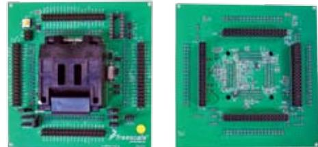
The cards include a CTI, Yamachi or Enflas zero insertion force (ZIF) socket, a background debug mode (BDM) connector and prototype connector ring. Configured for oscillator operation, the adaptor cards include support for a user supplied clock oscillator. They are compatible for use with any BDM tool.
