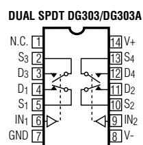
SWITCH STATES ARE FOR LOGIC "1" INPUTS (POSITIVE LOGIC).
