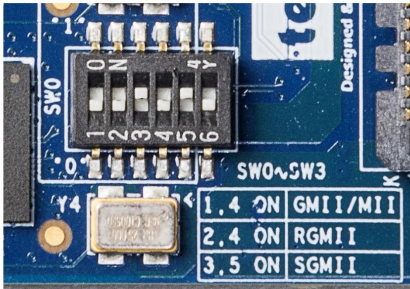
Figure 2-7 SW0 setting for ETH0 port SGMII mode
