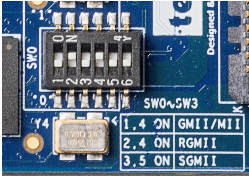
Figure 2-5 SW0 setting for ETH0 port RGMII mode
