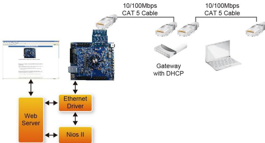
Figure 4-1 hardware setup of remote-update portal demonstration
