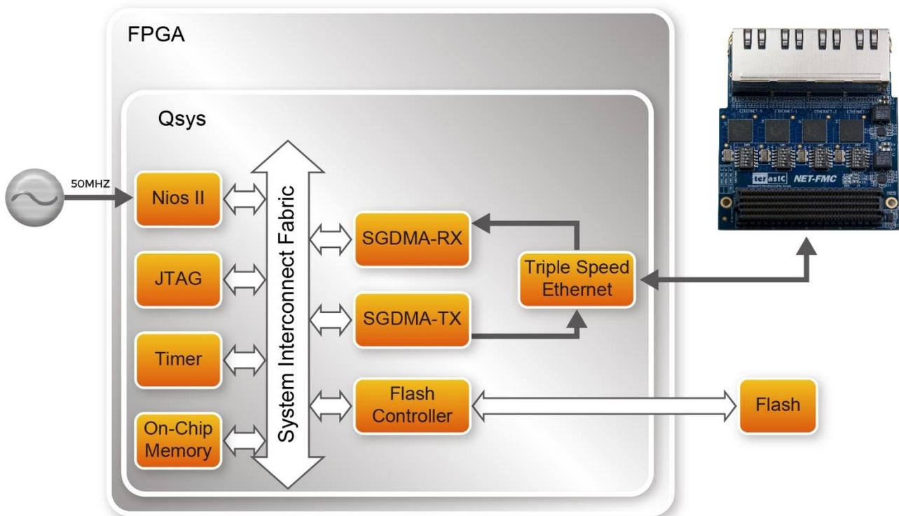
Figure 4-2 Function block diagram of remote-update portal demonstration
