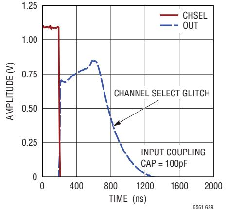
**Pulse Stretching  $C_{IN} = 0.5\text{pF}$ ,
