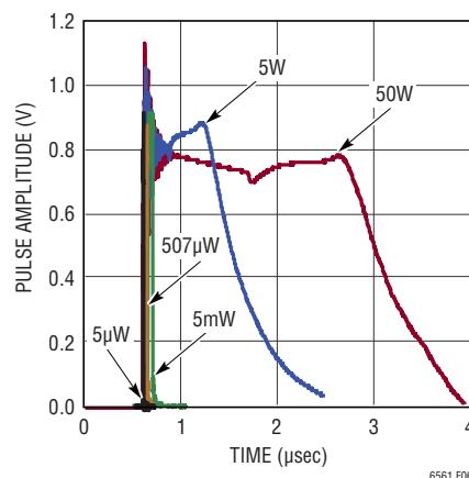
Figure 10. Pulse Width vs Input Hi Power Optical
