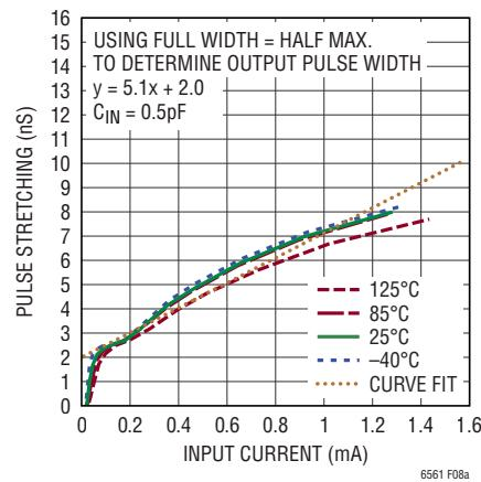
Figure 8a. Pulse Stretching  $C_{IN} = 0.5\text{pF}$ , Using FWHM
