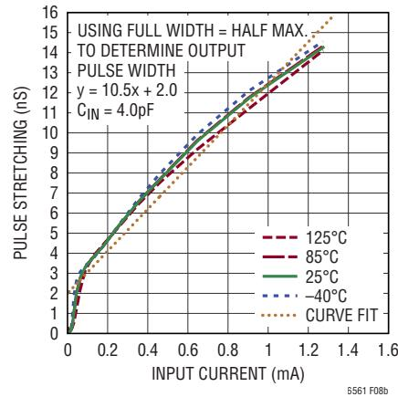
Figure 8b. Pulse Stretching  $C_{IN} = 4\text{pF}$ , Using FWHM
