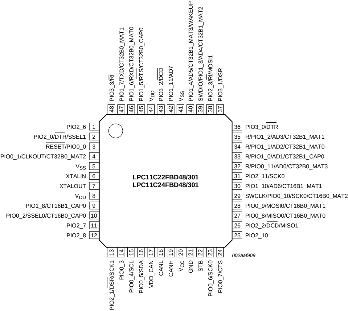
Fig 3. Pin configuration (LPC11C22/C24)
