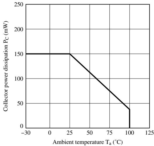
**Fig.5 Total Power Dissipation vs. Ambient Temperature**
