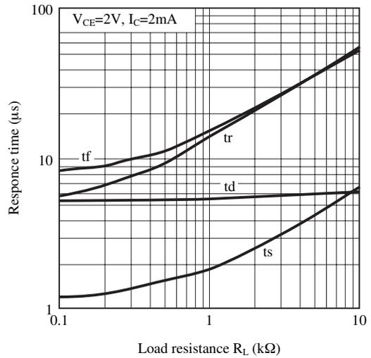
**Fig.14 Response Time vs. Load Resistance (Saturation region)**
