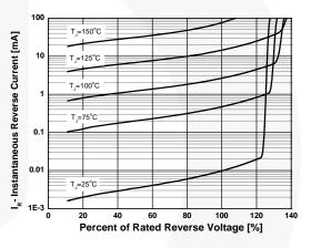
Figure 3. Typical Reverse Characteristics
