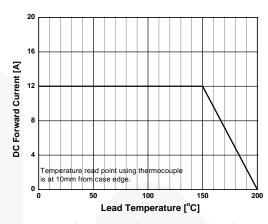
Figure 1b. DC Forward Current Derating Curve
