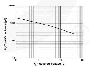
Figure 5. Typical Junction Capacitance
