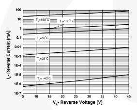
Figure 2. Reverse Current vs. Reverse Voltage
