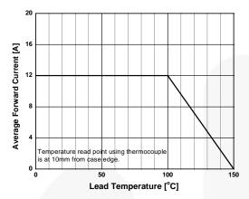
Figure 1a. Average Forward Current Derating Curve
