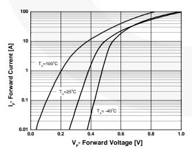
Figure 4. Forward Voltage vs. Forward Current
