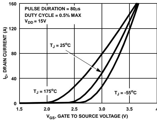
**Figure 7. Transfer Characteristics**
