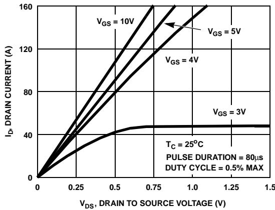
**Figure 8. Saturation Characteristics**
