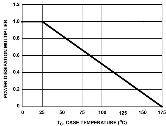
Figure 1. Normalized Power Dissipation vs Case Temperature
