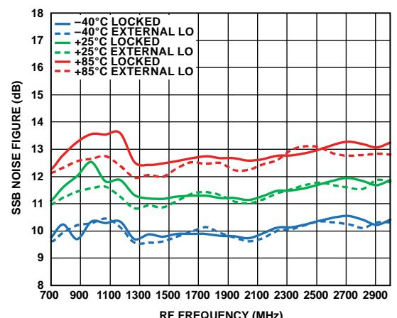
Figure 9. SSB Noise Figure vs. RF Frequency over Three Temperatures
