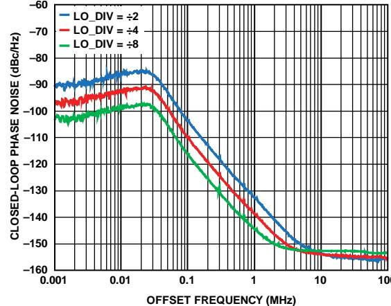
Figure 63. VCO\_0 Closed-Loop Phase Noise vs. Offset Frequency for Various
