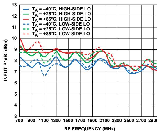
Figure 58. Input P1dB vs. RF Frequency over Three Temperatures
