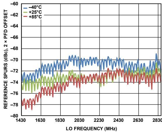
Figure 93.  $f_{PFD}$  Reference Spurs vs. LO Frequency,
