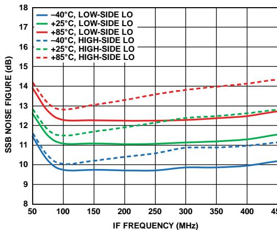
Figure 21. SSB Noise Figure vs. IF Frequency for Three Temperatures
