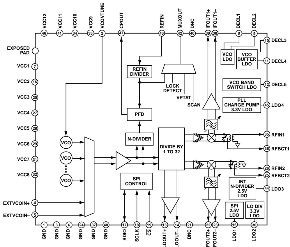
Figure 110. Simplified Schematic
