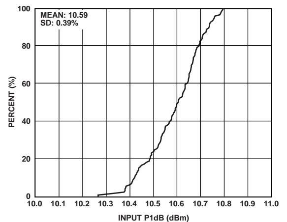
Figure 33. Input P1dB Distribution
