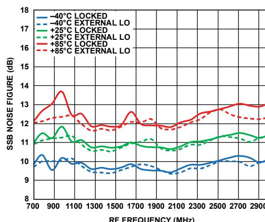
Figure 59. SSB Noise Figure vs. RF Frequency over Three Temperatures
