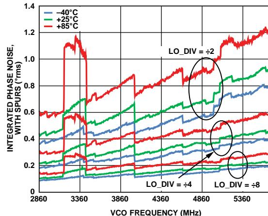
Figure 81. 10 kHz to 40 MHz Integrated Phase Noise vs. VCO Frequency, Divide by Two, Four, and Eight, Including Spurs
