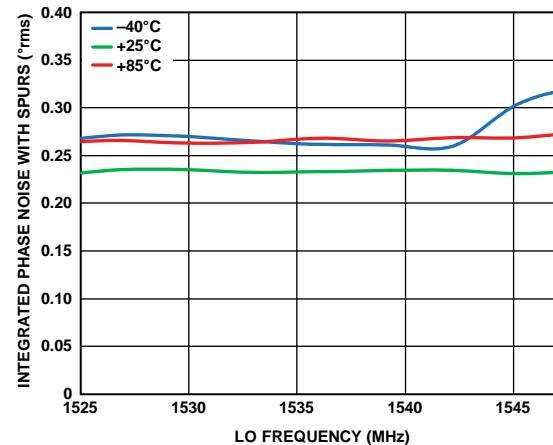
Figure 82. VCO\_4 10 kHz to 40 MHz Integrated Phase Noise vs. VCO Frequency, For Various Temperatures, Including Spurs
