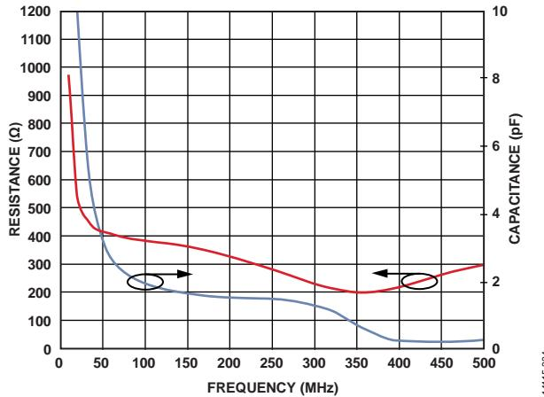
Figure 34. IF Output Impedance (R Parallel C Equivalent)
