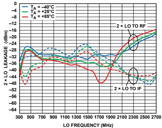
Figure 27.  $2 \times$  LO Leakage vs. LO Frequency over Three Temperatures ( $2 \times$  LO to RF and  $2 \times$  LO to IF)
