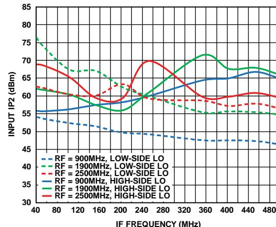
Figure 19. Input IP2 vs. IF Frequency for Three RF Frequencies
