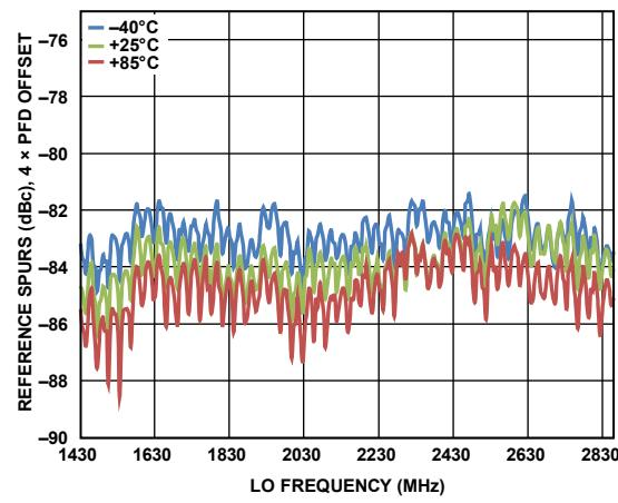
Figure 95.  $f_{PFD}$  Reference Spurs vs. LO Frequency,
