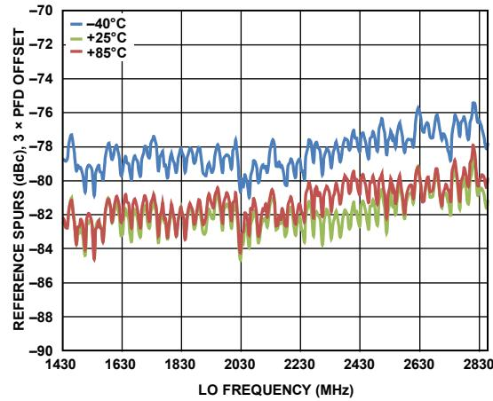
Figure 94.  $f_{PFD}$  Reference Spurs vs. LO Frequency,
