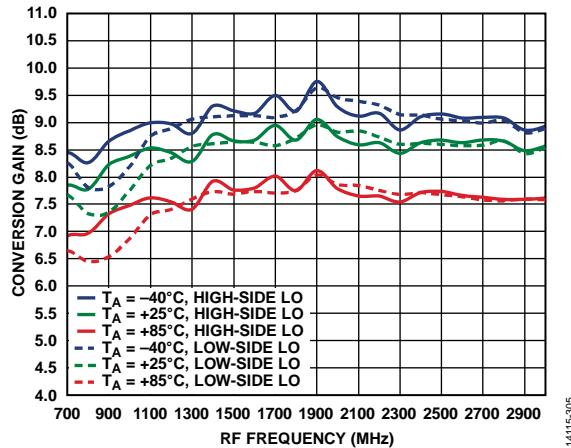
Figure 5. Power Conversion Gain vs. RF Frequency over Three Temperatures,
