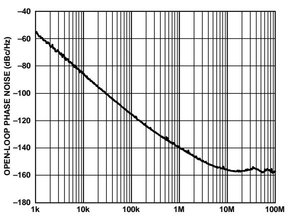
Figure 62. VCO\_2 Open-Loop Phase Noise vs. Offset Frequency,
