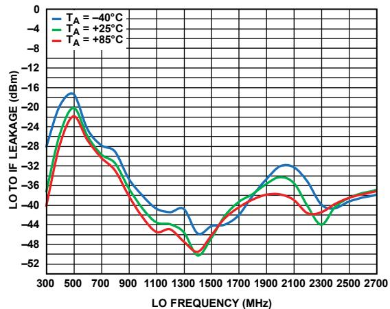
Figure 25. LO to IF Leakage vs. LO Frequency over Three Temperatures
