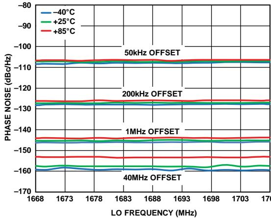
Figure 83. VCO\_5 GSM Loop Filter Phase Noise, Divide by Two Selected, Offset = 50 kHz, 200 kHz, 1 MHz, and 40 MHz
