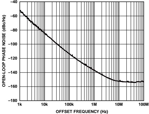
Figure 60. VCO\_0 Open-Loop Phase Noise vs. Offset Frequency,
