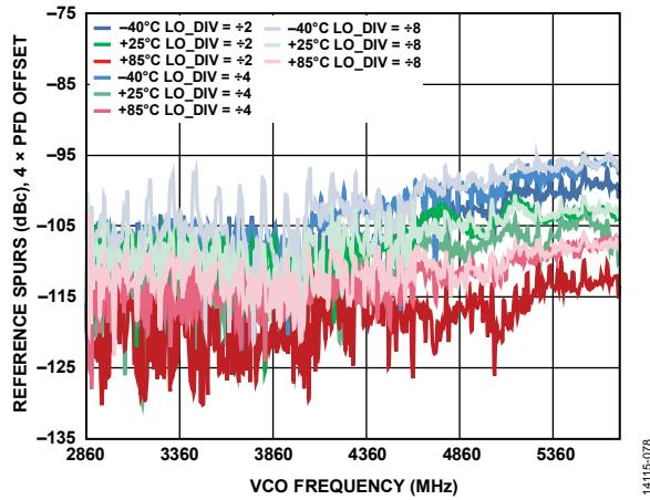
Figure 90.  $f_{PFD}$  Reference Spurs vs. VCO Frequency,
