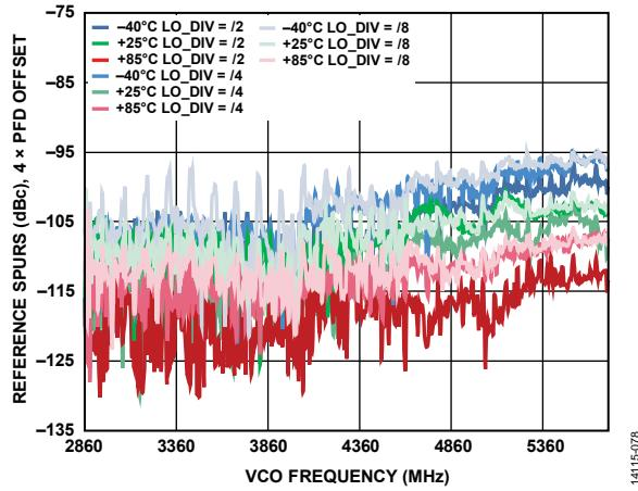
Figure 91.  $f_{PFD}$  Reference Spurs vs. VCO Frequency,
