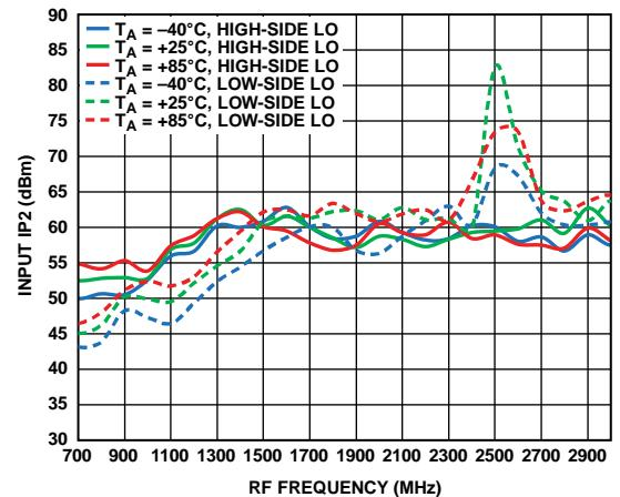
Figure 7. Input IP2 vs. RF Frequency over Three Temperatures
