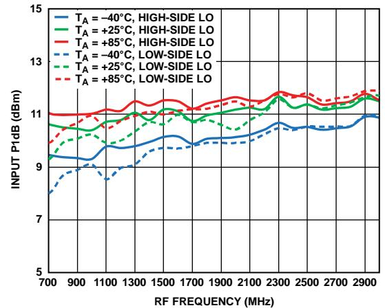
Figure 8. Input P1dB vs. RF Frequency over Three Temperatures
