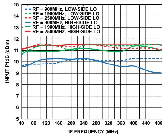
Figure 20. Input P1dB vs. IF Frequency for Three RF Frequencies
