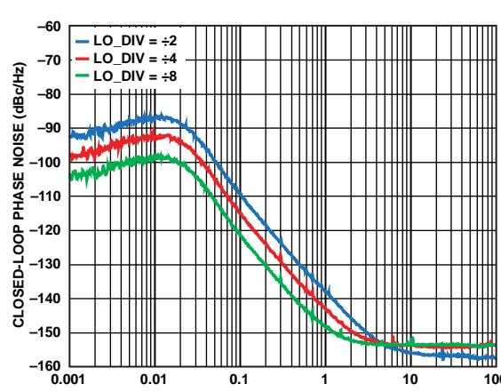
Figure 65. VCO\_2 Closed-Loop Phase Noise vs. Offset Frequency for Various
