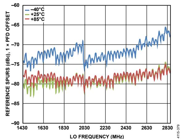
Figure 92.  $f_{PFD}$  Reference Spurs vs. LO Frequency,
