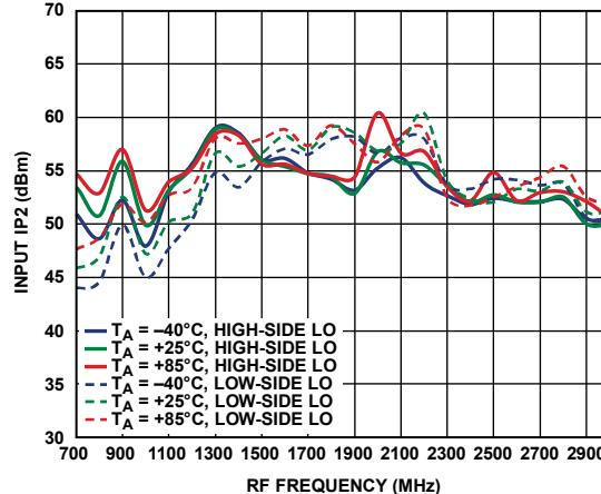
Figure 57. Input IP2 vs. RF Frequency over Three Temperatures
