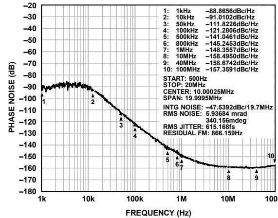
Figure 118. GSM Phase Noise Performance at 1.535 GHz
