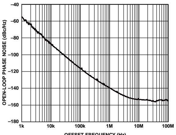
Figure 61. VCO\_1 Open-Loop Phase Noise vs. Offset Frequency,
