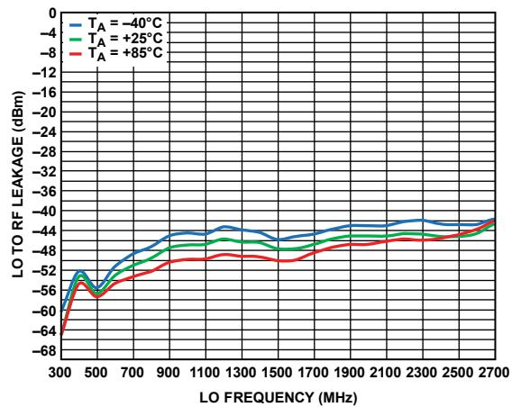
Figure 26. LO to RF Leakage vs. LO Frequency over Three Temperatures
