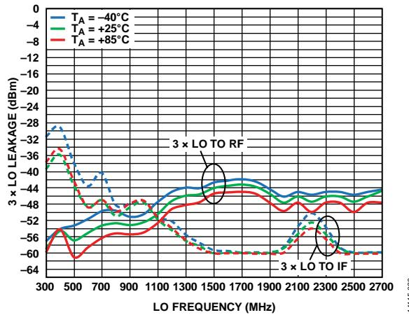
Figure 28. 3x LO Leakage vs. LO Frequency over Three Temperatures
