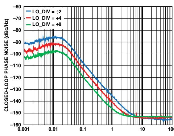
Figure 64. VCO\_1 Closed-Loop Phase Noise vs. Offset Frequency for Various
