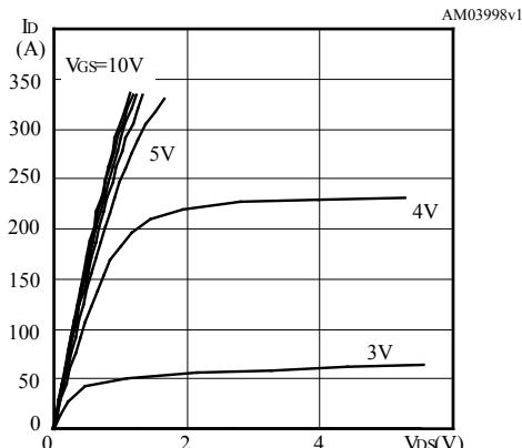
**Figure 4. Transfer characteristics**
