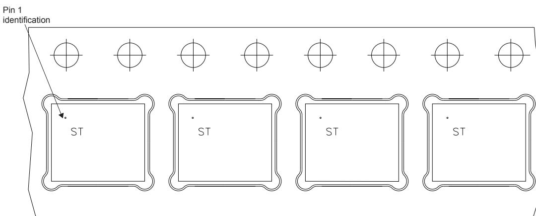
Figure 22. PowerFLAT™ 5x6 reel
